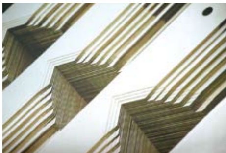
4阶叠缝技术 Ademonstration of 4-step-lap at joint area
